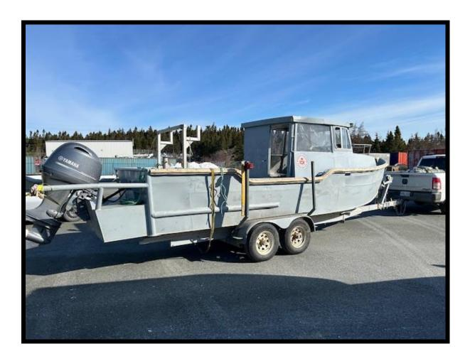
Pro-Dive owns a locally built aluminum hull utility boat that is utilized for marine work and to support diving operations as required.
